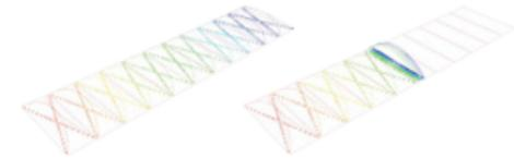
4. C# scripting within grasshopper provides more complex control over the arc position in the x axis. This allows the roof structure to translate to an open or closed position.
