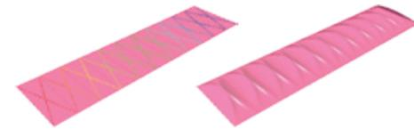
3. With provided custom python components, rail curves are created and the mesh is tweened into a form found position.
